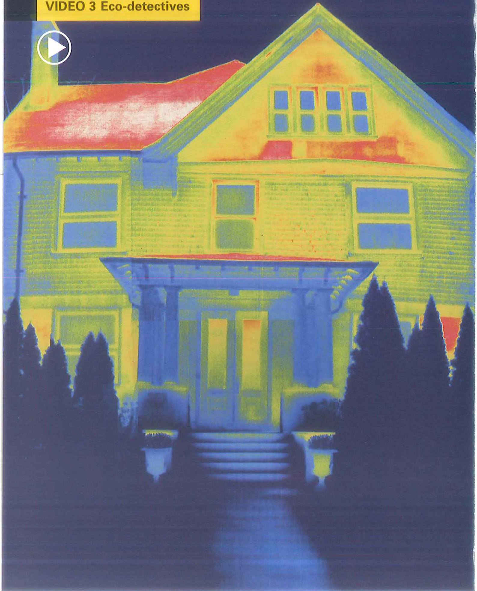
Heat loss through the walls of a house with poor insulation, New Haven, Connecticut
